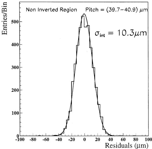
Fig. 7. Gaussian fit to the distribution of residuals and the intrinsic resolution for non inverted region.
