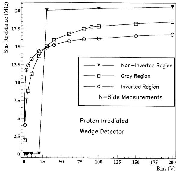
Fig. 5. Bias resistance vs. bias voltage in three different regions along the detector.
