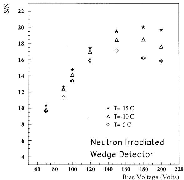
Fig. 4. Signal-to-noise ratio vs. bias voltage after neutron irradiation at  $T = -5^{\circ}\text{C}$ ,  $-10^{\circ}\text{C}$ ,  $-15^{\circ}\text{C}$ .
