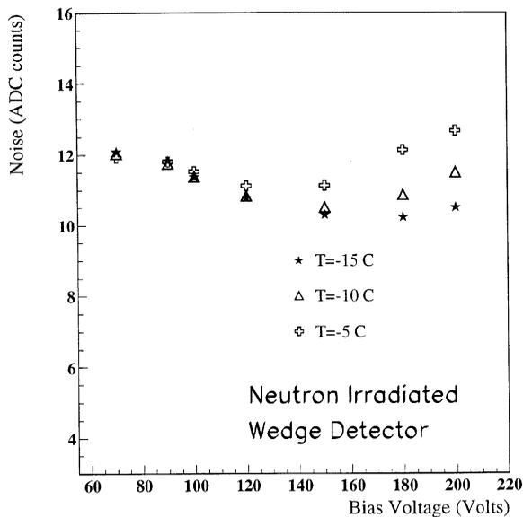
Fig. 2. Mean value of cluster noise vs. bias voltage, at  $T = -5^{\circ}\text{C}$ ,  $-10^{\circ}\text{C}$ ,  $-15^{\circ}\text{C}$ .
