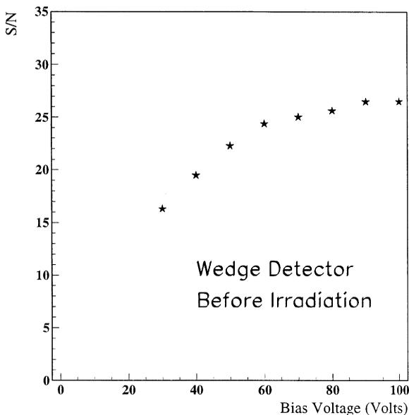
Fig. 3. Signal-to-noise ratio vs. bias voltage before neutron irradiation at  $T = 20^{\circ}\text{C}$ .
