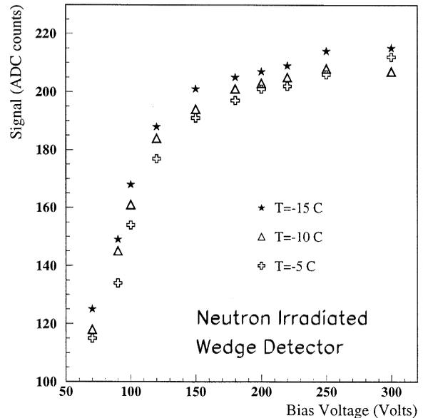
Fig. 1. Most probable value of collected charge (from Landau curve fit to the data) vs. bias voltage, at  $T = -5^\circ\text{C}$ ,  $-10^\circ\text{C}$ ,  $-15^\circ\text{C}$ .
