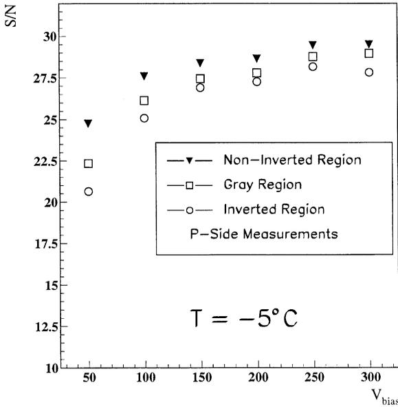
Fig. 6. Signal-to-noise ratio vs. bias voltage in three different regions along the proton irradiated detector.
