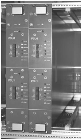
Figure 3: Two power supply modules lodged in the crate
