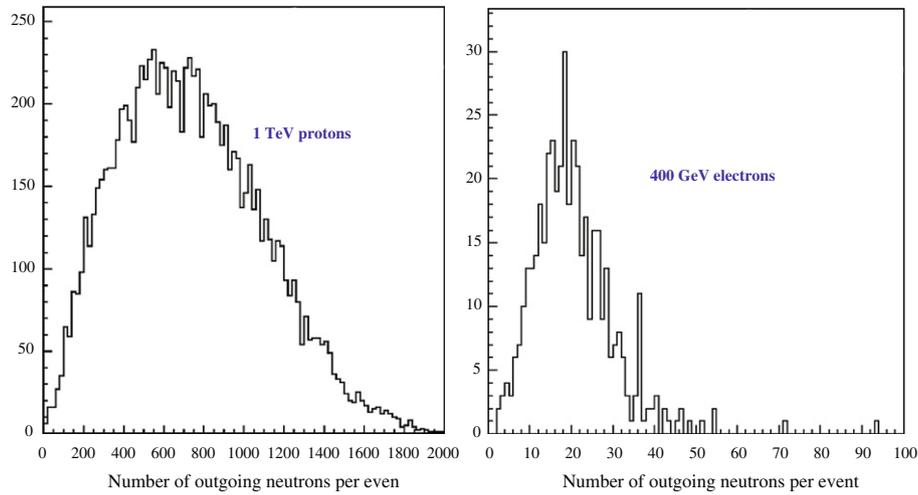
Fig. 1. Neutron yield outside the CALET calorimeter for 1 TeV interacting protons and 400 GeV electrons.
