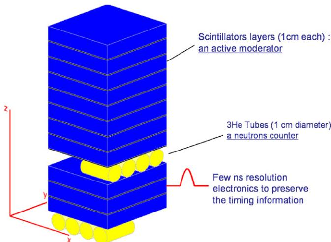
Fig. 3. A scheme of the proposed NEUCAL neutron detector.
