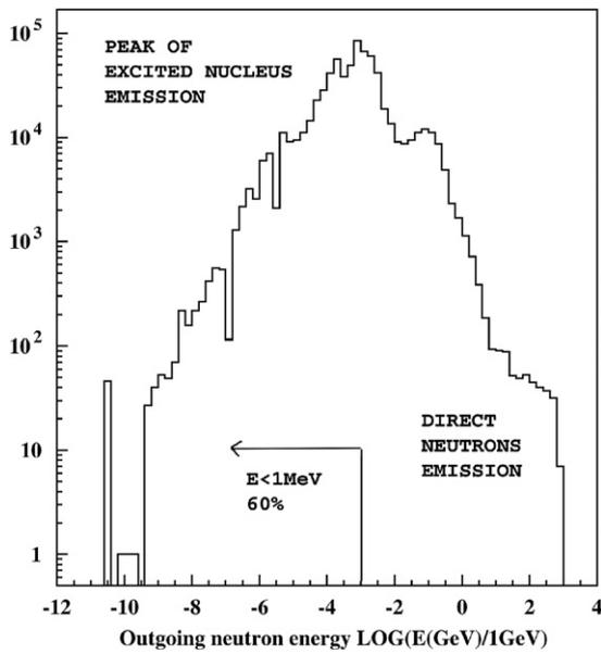
Fig. 2. Energy distribution of neutrons exiting from the CALET calorimeter in case of 1 TeV interacting protons.
