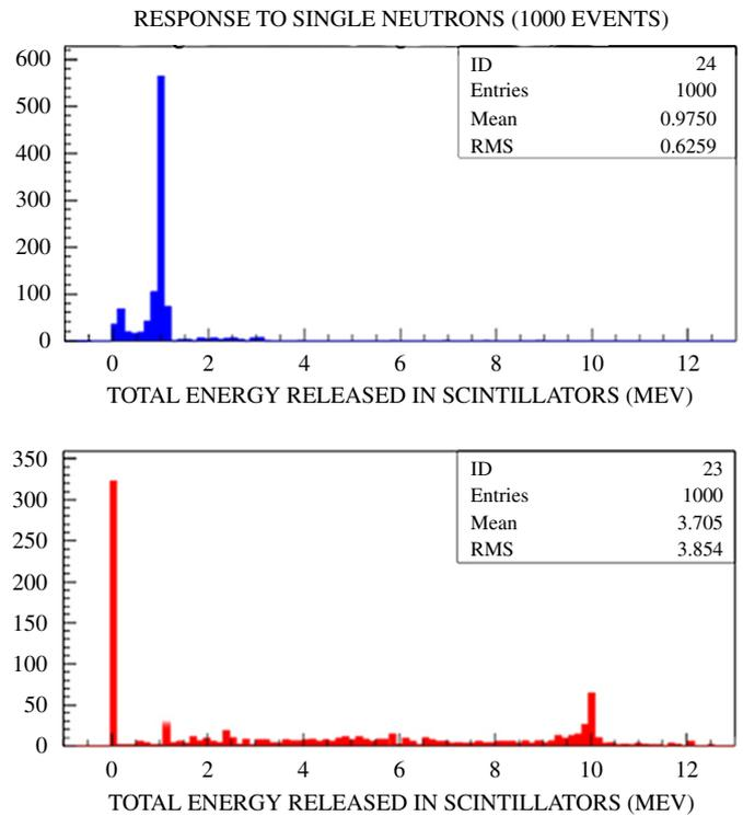
Fig. 4. Response of 12 scintillator layers to single neutron. The figure on top shows the energy released in all the scintillators by 1 MeV neutrons. The figure on the bottom refers to the response in case of 10 MeV neutrons.
